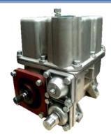
VP80G is a self-priming gear type suction unit with a certified gas separator, adjustable sealed bypass valve, control valve and washable stainless steel inlet filter. VP80G works silent with proven performance in the harshest conditions. VP120 is a self-priming vane type suction unit with the same functionalities for heavy duty applications.
