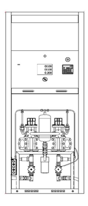
Mekser know-how and benefits in a compact package. Using galvanized steel as a start, electrostatic powder coating provides strong protection against wide range of weather conditions. Stainless steel option for ultimate protection against extreme conditions including salty environments by ocean.
