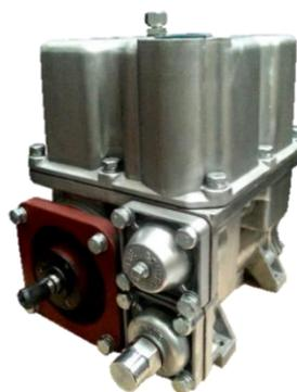
VP80G is a self-priming gear type suction unit with a certified gas separator, adjustable sealed by-pass valve, control valve and washable stainless steel inlet filter. VP80G works silent with proven performance in the harshest conditions. VP120 is a self-priming vane type suction unit with the same functionalities for heavy duty applications.
